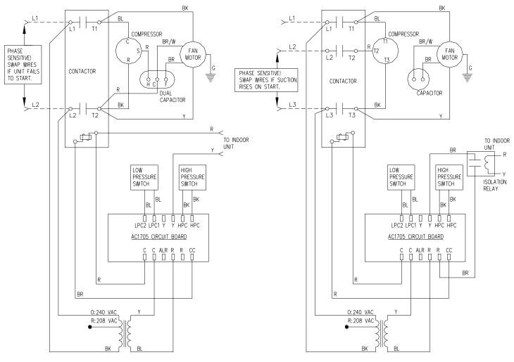
$\underline{\chi}$  WARNING: CORRECT POLARITY REQUIRED. IF UNIT FAILS TO START PROPERLY, SWAP POWER WIRES.
