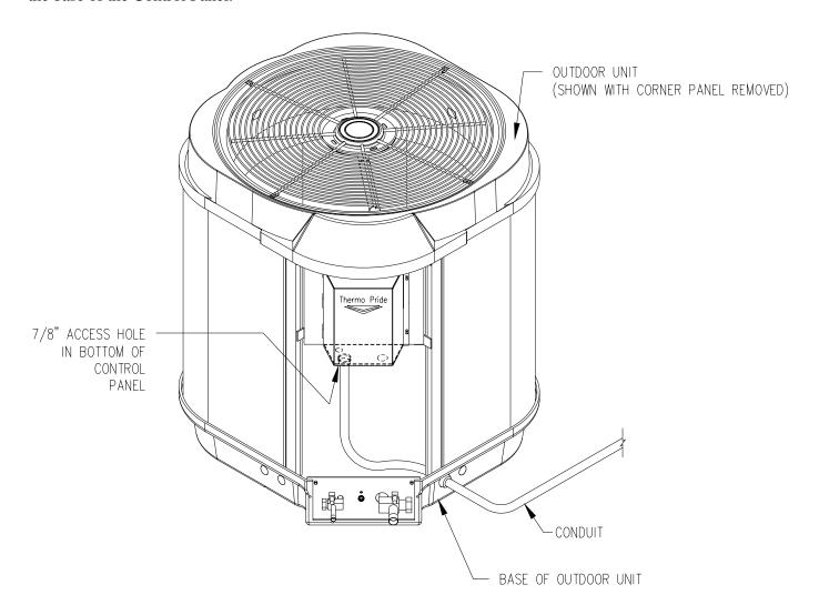
Reference Table A for unit electrical characteristics. Bring proper service to the unit through a circuit breaker or fused disconnect switch, in accordance with local codes. In the case of a single phase 230 VAC unit, the neutral wire should be brought to the unit in order to provide ground service. A ground wire must be connected to the unit at the screw or pressure connector marked "ground".
