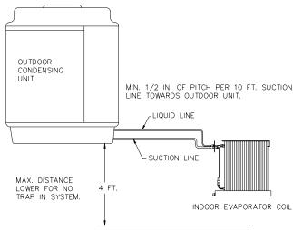
2. A trap is necessary in the suction line at the indoor evaporator coil if the indoor evaporator coil is more than 4' below the outdoor condensing unit and 1 trap per every 10' of vertical rise thereafter.
