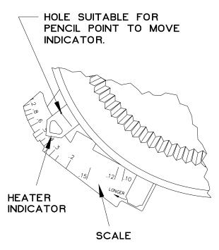
Figure 5: Heat Anticipator Adjustment Scale
