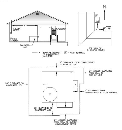
Figure 1: Selection of Appliance Installation Location
