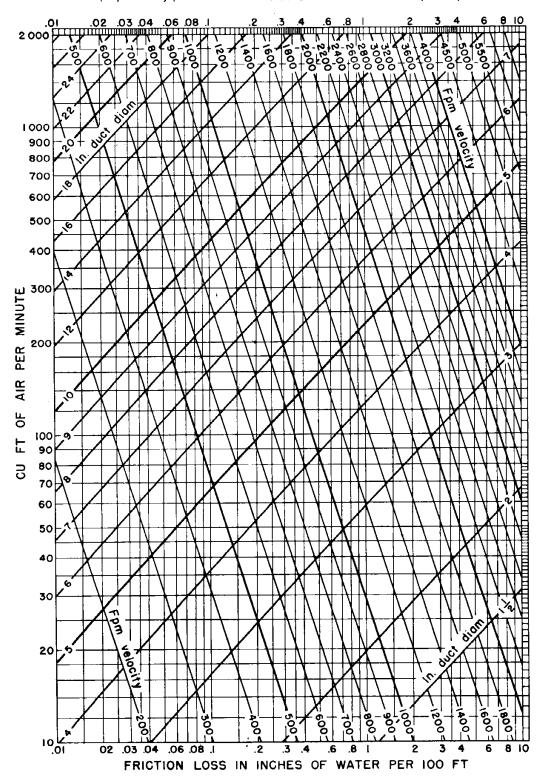
(Based on Standard Air of 0.075 lb per cu ft density flowing through average, clean, round, galvanized metal ducts having approximately 40 joints per 100 ft.) Caution: Do not extrapolate below chart.
