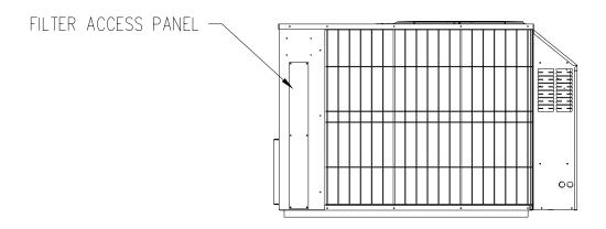
Figure 12: Location of the OPB Supply/Return Air Filter
