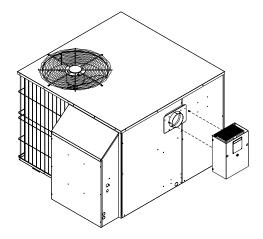
**FIGURE 2: Vent Terminal Mounting Position**
