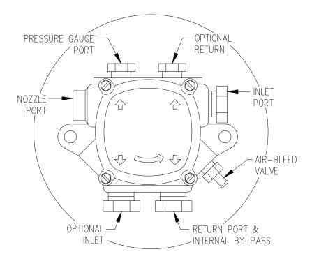
Figure 13: Location of Oil Pump Vent Plug
